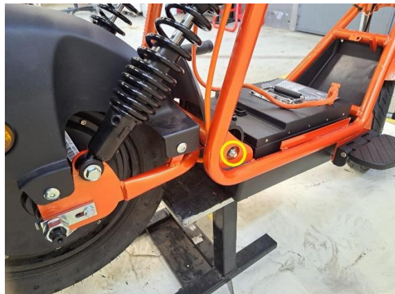
Irrota takahaarukan akselipultin lukitusmutteri (hylsy 14 mm, 12 mm).
